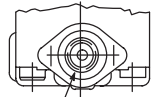
V2020P SECONDARY OUTLET PORT .875 14 UNF 2B STR. THD. SAE O-RING BOSS CONNECTION
