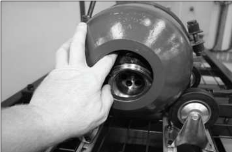
11. Remove as much air as possible from the Bladder, then remove the bladder from the Shell - do not use any sharp objects that could damage the bladder.
