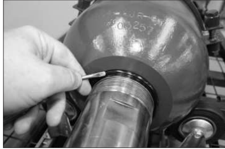
8. Holding the Fluid Port Body firmly install the metal back-up ring and the O-Ring. Ensure no sharp tools are used and that the O-Ring is inserted evenly around the Fluid Port Body.
