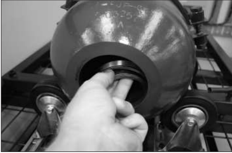
7. Grip the Fluid Port Body from inside the Shell and pull out as far as possible.
