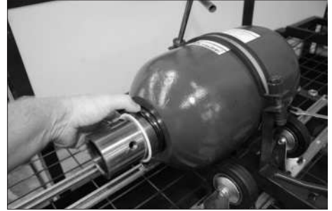
9. Ensuring the Fluid Port Body does not get dislodged - insert the Nylon Back-Up washer so that the rounded face on the washer faces the O-Ring.
