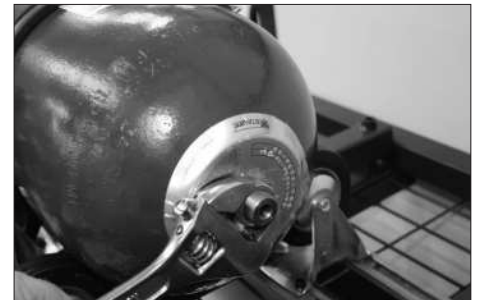
6. Remove the Bladder Lock Nut and Name Plate.
