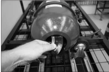
10b. From inside the shell slide the Anti extrusion ring off the Fluid Port body and remove from the shell.
