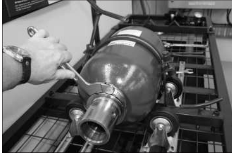
8. Remove the Fluid port Lock Nut with an appropriate "C" spanner along with the flanged washer.
