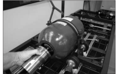
10c. The Fluid Port can then be removed from the shell.
