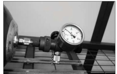
3. Attach STAUFF pre-charging head and release any pre-charge from the Accumulator.
