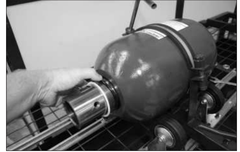
9. Remove the Nylon Back-up Washer and the metal back-up ring along with the O-Ring.
