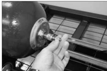
2. Remove the Gas Valve Assembly Cap.
